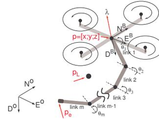
Fig. 1. QM system with  $m$ -DOF arm:  $p = [x; y; z]$  is quadrotor platform’s center position,  $p_e = [x_e; y_e; z_e]$  the end-effector position,  $\lambda$  the thrust force input and  $p_L$  is the center-of-mass position of the total QM-system.
