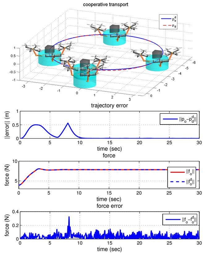
Fig. 5. Snapshots of the object transport using cooperative QM systems control of compliant behavior with unknown mass and parameter adaptation.
