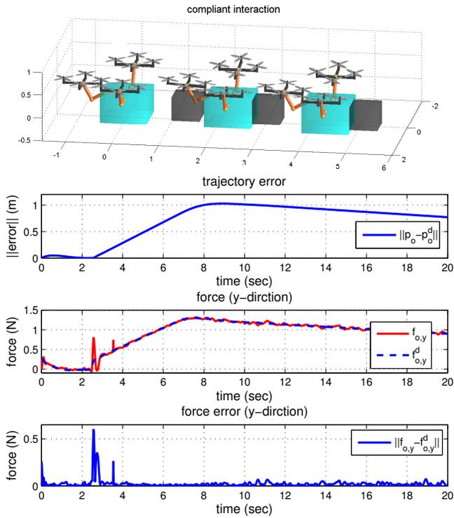
Fig. 4. Snapshots of the object pushing task using the multiple QM system under admittance-type force control with force profile.
