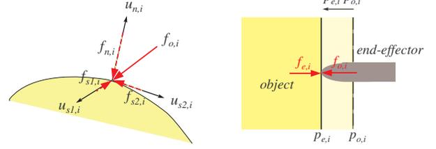
(a) Contact force decomposition (b) Object stiffness model
