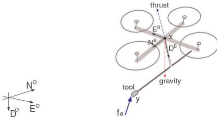
Fig. 1. Quadrotor with a tool
