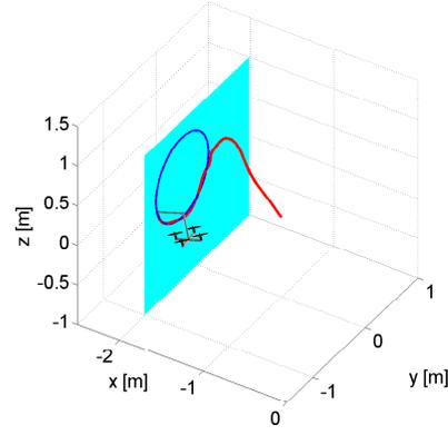
Fig. 2. Hybrid force/position control of quadrotor with a tool attached at  $d = [0.35; 0; -0.3]$  under the stabilizing  $\nu_3$ -action (26).
