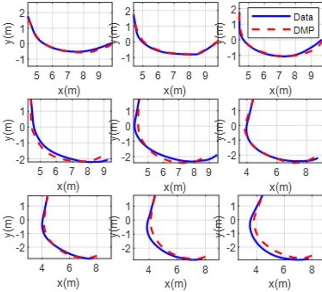
Fig. 6: Results of three times consecutive nominal trajectory retrieving in the training terrains from left to the right - top: flat terrain, middle: slope1, bottom: slope2
