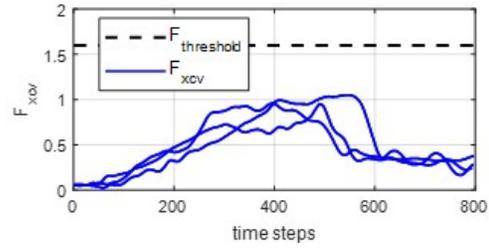
Fig. 10: External force data  $F_{xcv}$  during digging in flat terrain.
