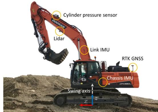
Fig. 1: Industrial autonomous robotic excavator, Doosan DX380LC, customized with IMUs, LiDAR, cylinder pressure sensor, RTK-GNSS sensors.
