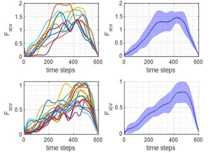
Fig. 7: Raw external force data from experts, resampling data, mean and variance between each data during excavation. Top: flat terrain, bottom: slope terrain
