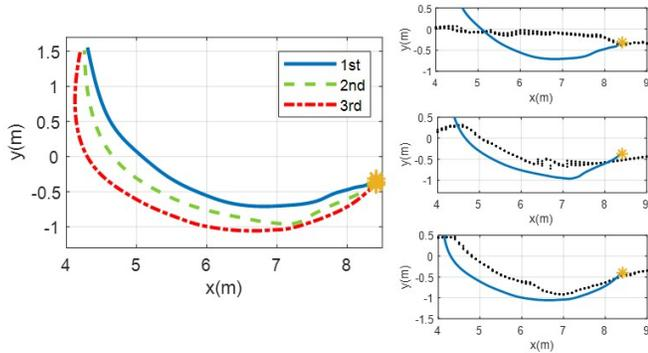
Fig. 9: Results of digging in flat terrain- left: plot of the three trajectories which operates deeper, right: each trajectory with  $y$ -dir flatten PCD before digging. The initial point is a yellow star.
