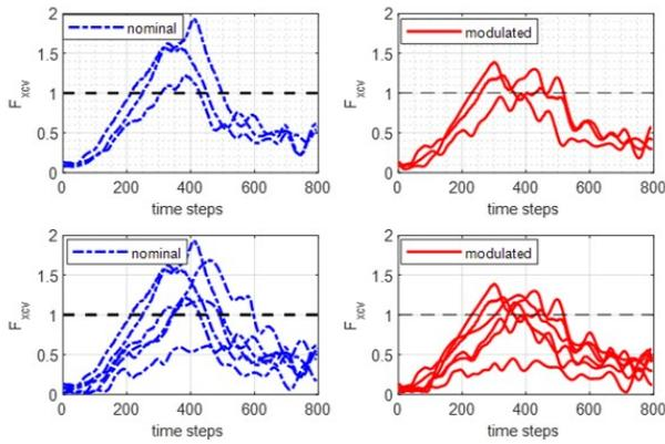
Fig. 12: External force results on slopes. The blue dotted lines are the results of the excavation force without feedback, and red lines are the excavation force results of considering coupling feedback. (top) slope 1, (bottom) slope 2.
