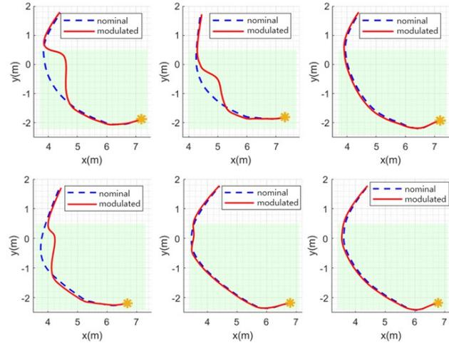
Fig. 11: Nominal trajectories and online modulating trajectories in slope 1 (top) and slope 2 (bottom) for consecutive three times excavations. The green area is digging inside the ground and the rest is booming up to designated goal point. The initial point is a yellow star.
