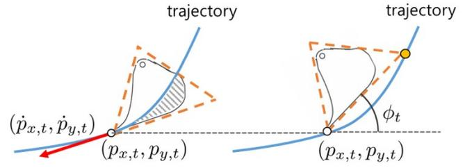
Fig. 5: Definition of bucket angle  $\phi$ . (left) The bucket tooth and headings coincide but the bucket collide with the ground. (right) The bucket tooth and headings form the minimum angle avoiding collision.
