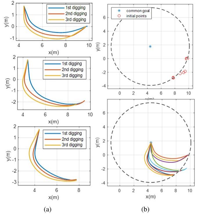
Fig. 3: The acquired expert excavation trajectories (eighteen data-set): (a) three rounds of consecutive excavation in flat and two different angled slopes; (b) modified training trajectory matching goal position  $y_g$  to equalize spatial scaling.
